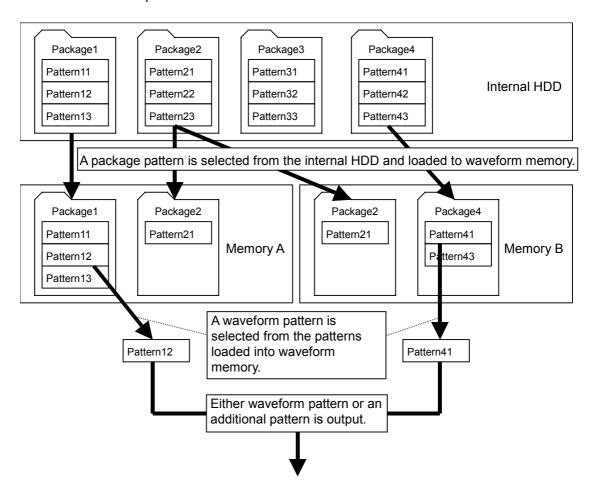
Refer to Section 3.5.2 "Using waveform pattern for modulation" in the MG3700A Operation Manual (Mainframe) for details on waveform pattern selection.
